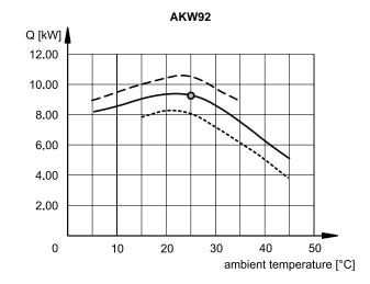
$H_2O$  temperature = ambient temperature  $H_2O$  temperature = ambient temperature +10 °C
