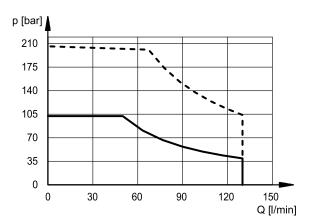
continuous operation ---- short-time operation (≤ 20% of duty cycle time)
