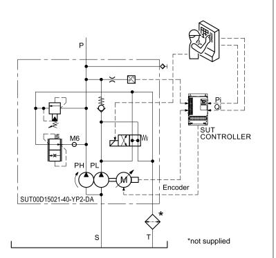
The flow is controlled during the cylinder operation. When the load pressure exceeds the pressure command, the rotation speed is reduced to control the pressure. The SUT allows bigger energy saving and more precise control of the machine, compared to conventional hydraulic control methods.
