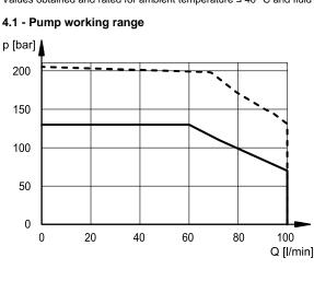
continuous operation → → → → short-time operation (≤ 20% of duty cycle time)
